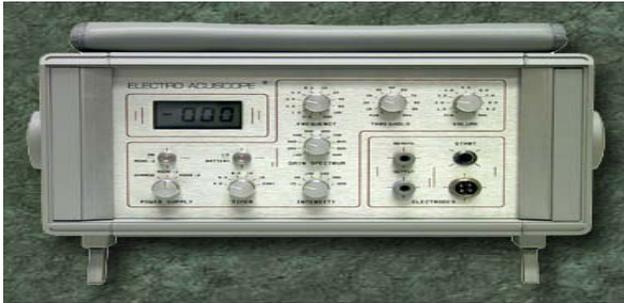
Fig. 2. An Electro-Acuscope used in measurement of pain level [4].
